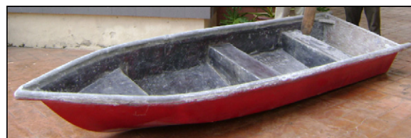
Fig. 5. Sugar palm fibre composite boat (Ishak, Sapuan, Leman, Sahari, & Ibrahim, 2010b).
